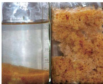
Untreated slurry (left) and MVP Frac slurry (right), immediately following agitation
