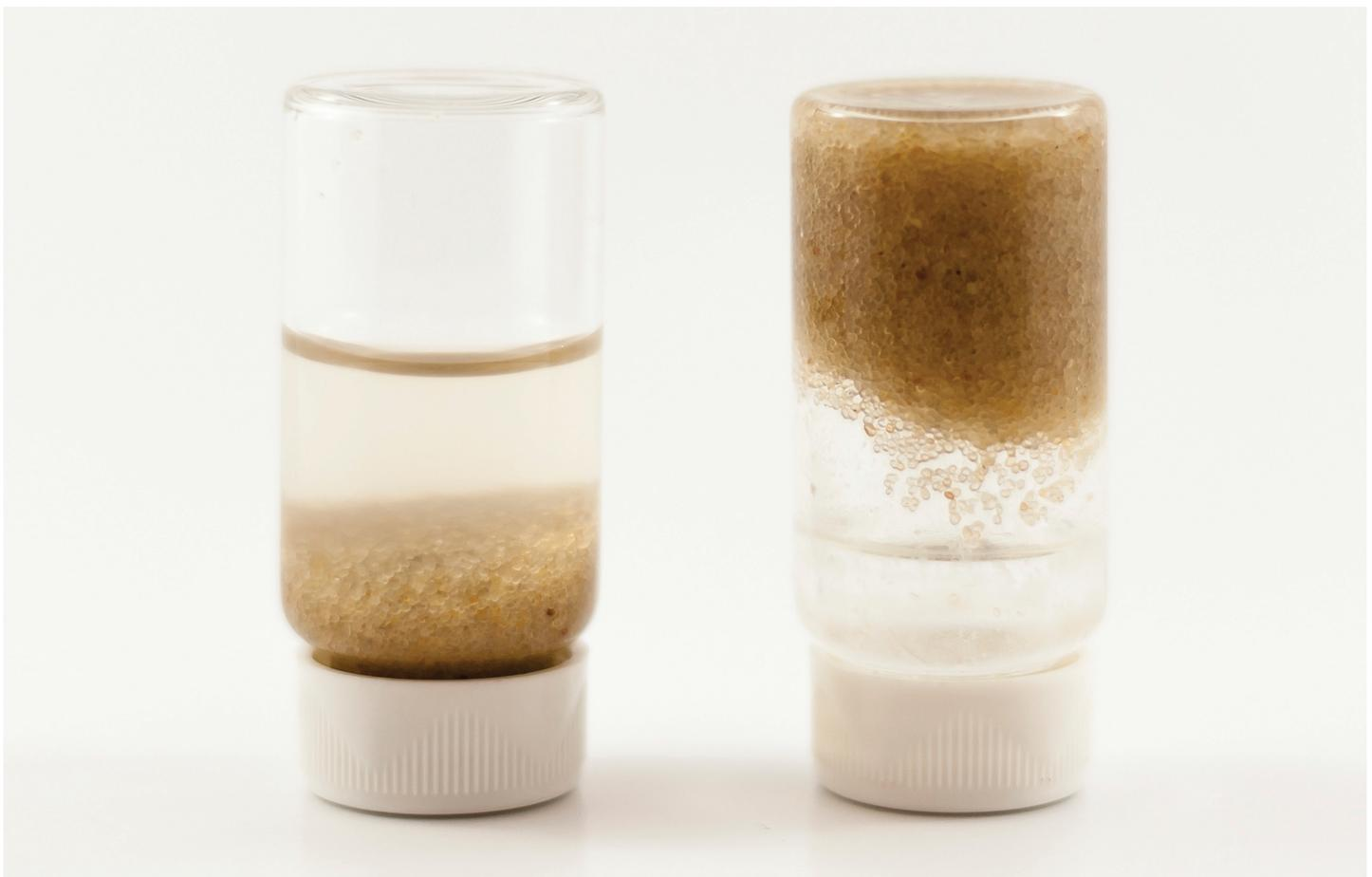
Untreated (left) and SandStill treated sand (right) in slick water
